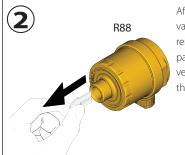
After the screwing of the R160 valve on the installation seat, remove the possible plastic paddle of the automatic air vent valve and proceed with the assembly.
