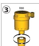
Screw the automatic air vent valve to the R160 valve, by making the plastic paddle be guided by the hole of the body of the automatic air vent valve.
