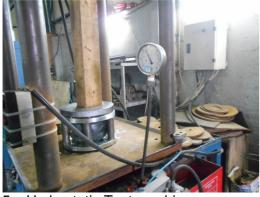
5. Hydrostatic Test machinery
