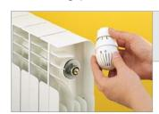
**1.** Open the head completely turning to this position .
